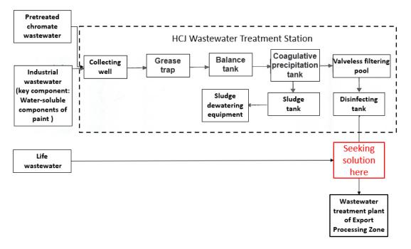
For now, most of the water currently being reused through the existing plants are used only for limited applications, such as gardening, toilets, and hangar washing. HAECO is looking for a wastewater solution that provides **higher quality water to be used for additional applications like hand washing, showering, and more.** The water does not need to be at the quality of drinkable.
