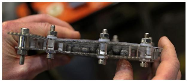
An iron-air cell at Form Energy in Somerville, a startup building massive batteries to store electricity produced by wind, solar, and other intermittent sources of renewable energy, on Feb. 15, 2022. DAVID L. RYAN/GLOBE STAFF
